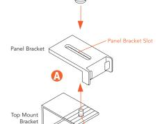
To create the top mount assembly, place panel brackets on top mount brackets, so that the top mount bolt fits into the panel bracket slot. Screw the thumbscrew onto
