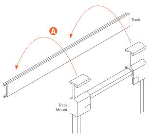
With the corner track mounts and track bumpers installed, place the VersaBoard onto the track.
